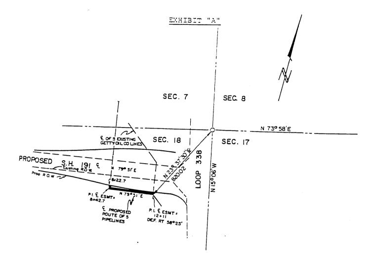
A CENTERLINE DESCRIPTION OF A GETTY PIPELINE IN SECTION 18, BLOCK 41, T-2-S, T & P RY CO SURVEY, ECTOR COUNTY, TEXAS.
